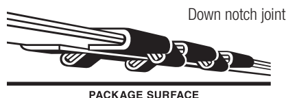
Down notch joint
