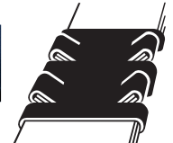
Reverse notch joint
